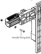
2. Tighten the hexagon nut+spring washer+inner lever with the designated tightening torque using a spanner with 10 mm width. If the inner lever is screwed loosely, it may result in product damage.
