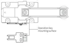
• Install the between bolt slide and guide aligning them within  $\pm 0.5$  mm from the center line. Excessive wear and damage on the product may result in trouble in operating the slide unit.
