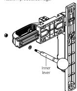
Tightening torque Inner lever 9 to 10 N·m
