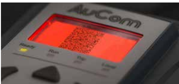
Dynamic QR codes allow easy access to useful operational data and event logs that are readable on your mobile device
