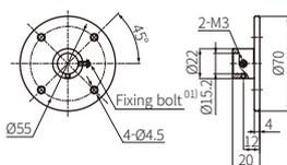
01) Recommended allowable tightening torque 0.5 ~ 0.9 N·m
